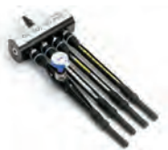
Adapter with Impactor connected in Dräger Aerotest Simultan
