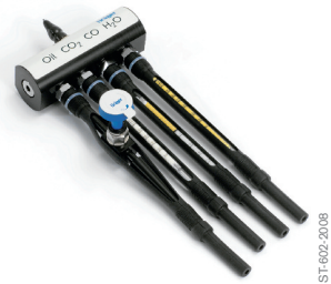
Impactor with Adapter in Aerotest Simultan
