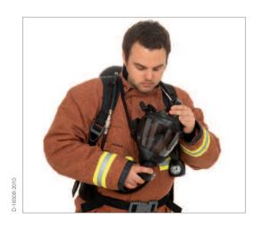
Reset lung demand valve by pressing red button in, taking care not to press centre of rubber cover.
