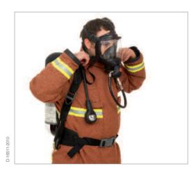
First breath will switch LDV to positive pressure mode, breathe normally. Inhale and hold breath – there must be no audible leak.
