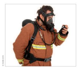
Close cylinder valve and breathe gently to exhaust air from system. Observe gauge, whistle will alarm at between 60 bar to 50 bar. Continue breathing down the system. Once empty, hold breath for approximately 3-5 seconds – the facemask should collapse and hold to face indicating a positive seal.
