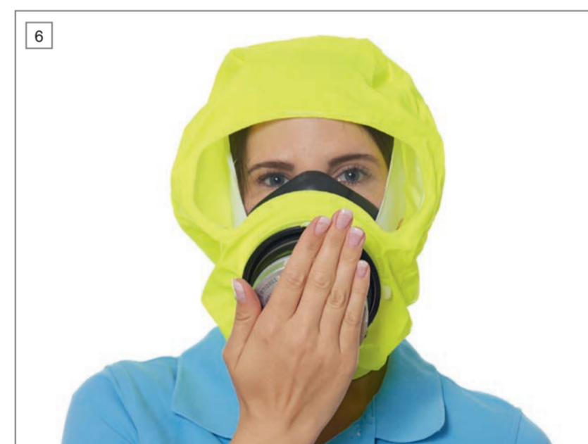
6 Check the fit of the half mask by closing the front filtering opening with the palm of your hand. If negative pressure is not generated readjust the half mask to ensure a close fit over nose and mouth.
